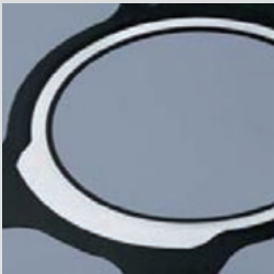
Removal of coating film from gasket
